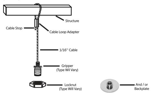
Insert Cable Into Bottom Of Loop Adapter And Pull Until Reaches Stop. Wrap Cable Around Structure
