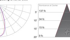
**C70 - 60 Degree** Delivered Light Output: 1387 Lumens Total Watts @120V: 17; Lumens Per Watt: 82 Center Beam Candle Power: 1377 Spacing Criteria: 1.06
