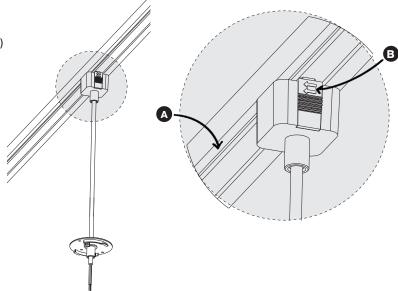
Attach the safety cable found inside of the Module to the Track Pendant Assembly and make the necessary connections.
