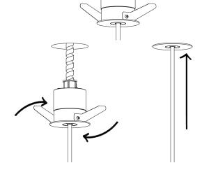
Attach the safety cable found inside of the module to the Micro Canopy assembly and make the necessary connections.
