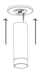
With the mounting tabs properly aligned, twist the module until the unit clicks into place (~20°).
