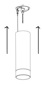
With the mounting tabs properly aligned, twist the module until the unit clicks into place (~20°).
