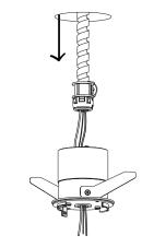
Attach conduit fitting to the topside of the Micro Canopy and install into the ceiling.
