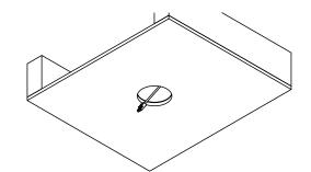
Pull driver output quick connect wiring through the aperture.
