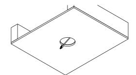
Pull driver output quick connect wiring through the aperture. Connect module to the driver output quick connect (A).
