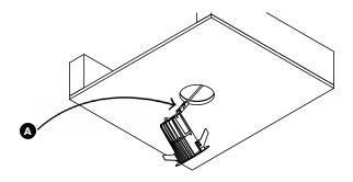
Compress leaf springs (B) to insert module into ceiling cutout. Twist module clockwise to help further engage the springs above the ceiling plane.
