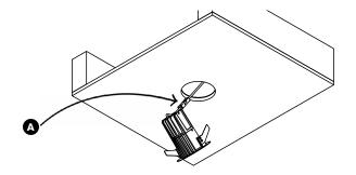
Compress leaf springs (B) to insert module into ceiling cutout. Twist module clockwise to help further engage the springs above the ceiling plane.
