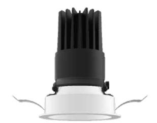
With a discreet 3" aperture, knife-edge trim and excellent visual cutoff - Lumenture's DLA75 blends discreetly into any environment. These recessed modules offer 35 degrees of tilt and deliver high lumens without glare. The result is superior brightness and quality from an unobtrusive fixture. DLA75 is available both in remodel with an attached junction box or with optional rough-in housings to fit any construction needs.
