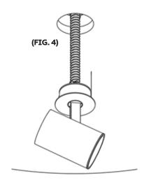
**STEP 5.** Compress springs and insert the canopy into the ceiling cutout until the trim is flush with the ceiling.
