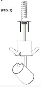
**STEP 4.** Once connections are made, replace cover and insert wiring compartment into the ceiling.
