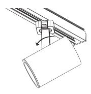
Fixture is fully connected when the adapter arrow is pointing towards the polarity line. You can now restore power to the track system!
